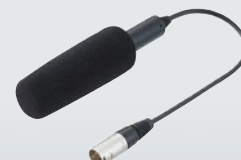
AG-MC200G XLR Microphone • Sensitivity: -40 dB ±3.5 dB (0dB=1V/Pa, at 1kHz) • Maximum Input level: 127 dB (1000Hz, Distortion within 1%) • S/N: More than 69 dB
