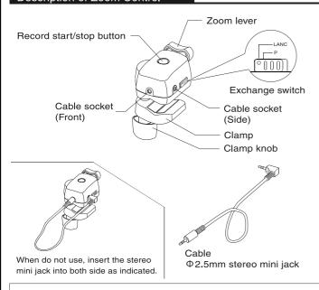
Clamp distance:  $\phi$  10mm(0.39inch) -  $\phi$  30 mm(1.18inch)
