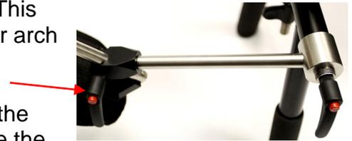
The tilt lever allows you to change the amount of tension in the tilting mechanism or soft-lock the tilt position. Never operate the Rig with the tilt lever excessively loose.
