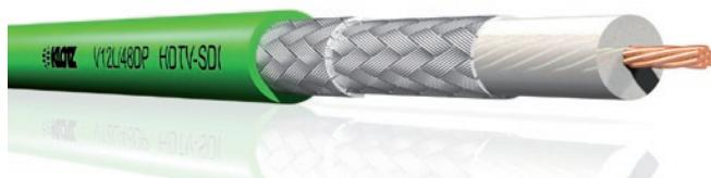
The universal video cable V12L48DP is optimally suited for the mobile transmission of HD-SDI and MADI signals. Due to the ultra-low signal attenuation transmission distances of over 100 meters are possible. The cable construction (flexible stranded inner conductor, two overlayed copper braids, extremely robust and abrasion-resistant outer jacket from PUR) is consequently designed for flexibility and robustness for mobile use on stage as well as outside.
