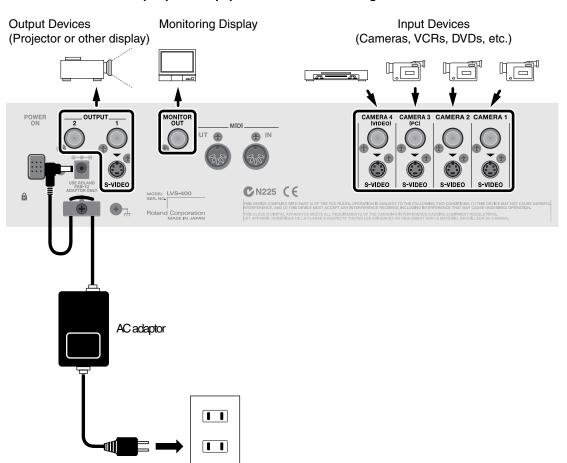
Connect the LVS-400 to peripheral equipment as shown in the figure.
