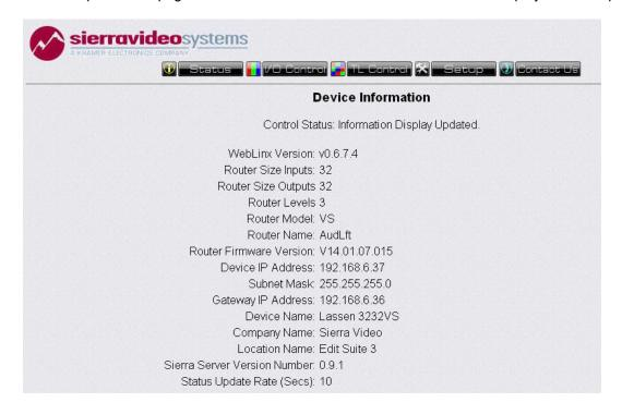
To setup IP address parameters, select "Setup".
