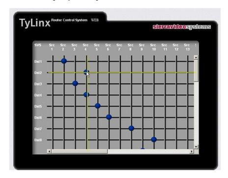
This screen displays a "grid" of sources and destinations. Left click on the I/O grid lines that intersect the source and destination to switch. Status is indicated by a blue dot at the I/O grid line.
