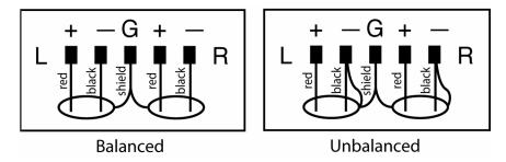
For unbalanced sources, connect the unbalanced source to one side of the balanced input and ground. The other input does not have to be grounded. Note, always use the same side of the balanced input for stereo.
