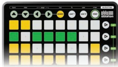
When Launchpad is chosen as an active control surface, a ring appears on the Session View to indicate which section is currently controlled by the pad matrix. Pressing a Clip Launch pad triggers the clip in the corresponding clip slot in Live. Hitting an empty clip slot in a track that is not armed will stop the clip playing in this track. If the track is armed to record, pressing the button records a new clip.
