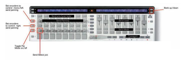
The left-hand ReMOTE ZeRO SL display will look as it does in Track mode however send routing is shown in place of abbreviated track names (the '-' symbol indicates no send routing):
