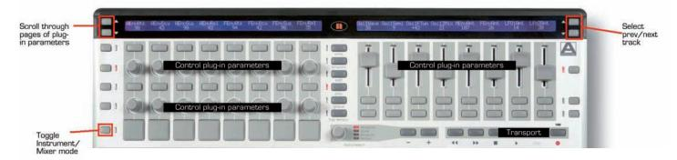
Note that only encoders, pots and sliders are used for control over plug-in parameters in Logic Instrument mode, not buttons.
