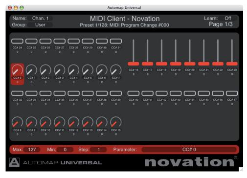
The default MIDI control map has 129 assigned controls across multiple pages. Each control is assigned to a different MIDI Control Change (CC) number, starting from O and going up to 127, plus an extra control at the end assigned to pitch bend. This is how the controls will be mapped when you activate a MIDI channel, however you can change the default MIDI control map by reassigning the controls and using the 'Set As Default' option.
