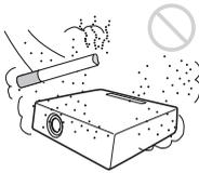
Avoid installing the unit in a very dusty or extremely smoky environment. Otherwise, the air filter will become obstructed, and this may cause a malfunction of the unit or damage it. Dust preventing the air passing through the filter may cause a rise in the internal temperature of the unit. Clean the air filter whenever you replace the lamp.
