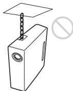
Use the Security bar at the side of the projector for a purpose of preventing theft, by attaching a commercially available theft prevention cable for example. If you lift the projector by holding the Security bar, or hang the projector by using this bar, it may cause the projector to fall or be damaged.
