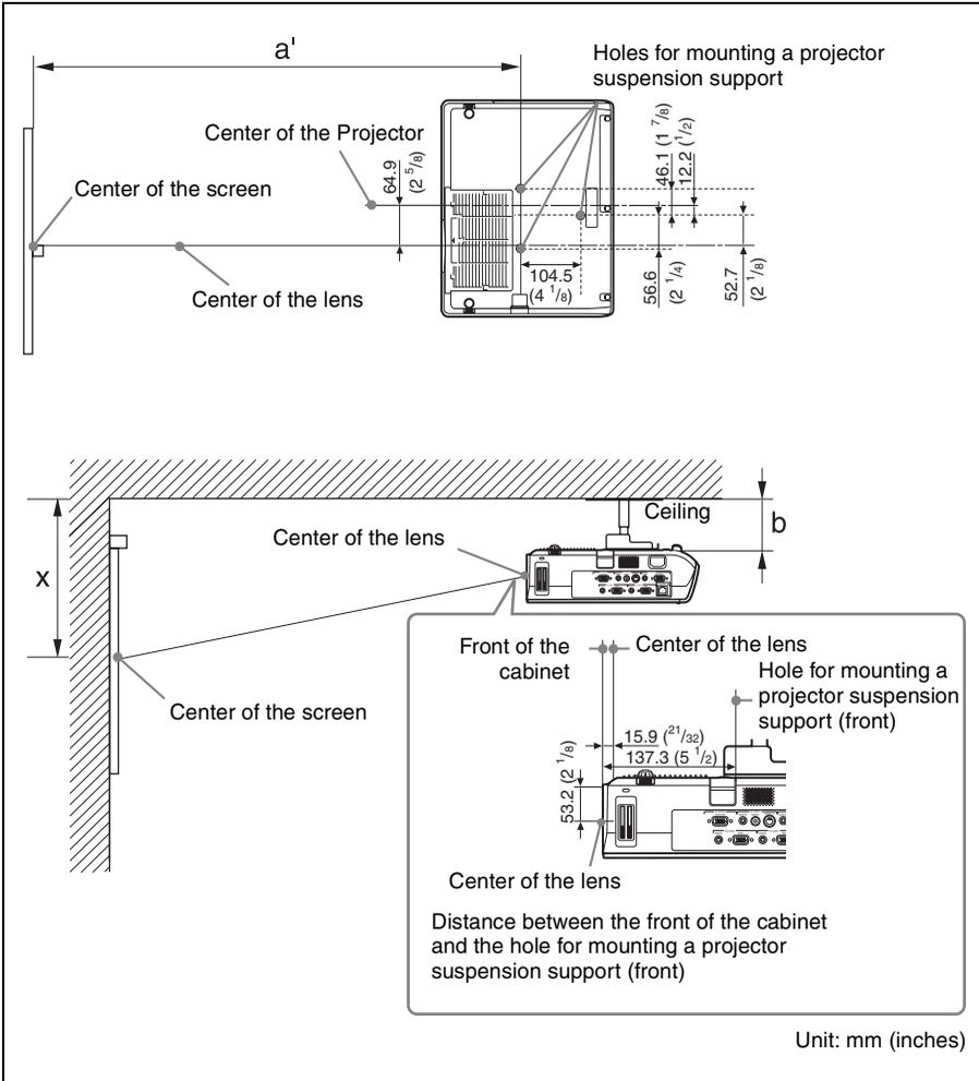
This section describes the examples for installing the projector on the ceiling.
