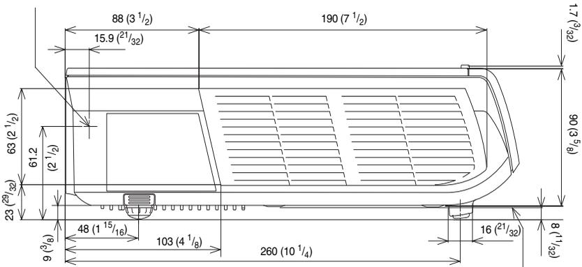
Projector suspension support mounting surface
