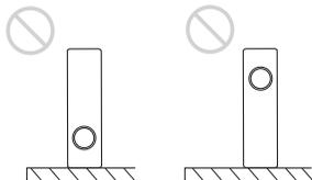
Avoid using as the unit topples over on its side. It may cause malfunction.
